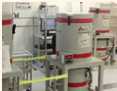
Inspection by germanium semiconductor detector (Fukushima Agricultural Technology Center laboratory)
